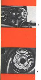
The battery case is mounted externally, so that cell replacement can be carried out on a loaded camera, without risk of spoiling the film. Proceed as follows: unscrew the cap (E), remove the spent cells and replace with new ones. Make sure that the cells are inserted correctly—i.e., "+" side towards the cap.
